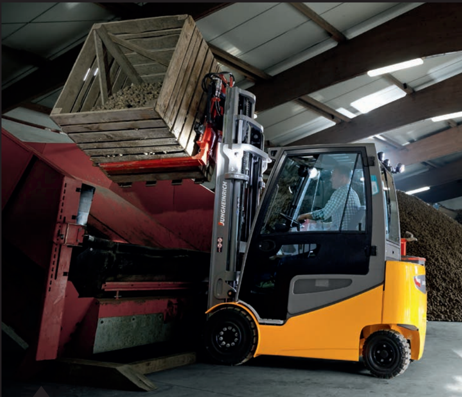
EFG 425k with a special rotating device.
